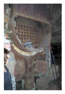
This is the boiler that provided the steam power for the carriage and saw blades in the main part of the mill. Once a week some unlucky 'small' person had to climb in the hole in the center and clean out the debris, which was considerable.
