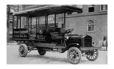
By 1912, the Commercial Trucks grew in size with more horsepower adding in a 2 cylinder engine. That's when they introduced the three-speed sliding gear transmission which was adopted using three-point mounting on a subframe and moving the engine to the front of the trucks with the clutch type being a leather-faced cone.
