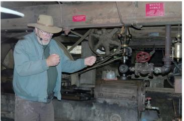
Our docent explaining the workings of the Atlas 30HP 200 RPM engine that drove the carriage....that's the widget that moves the logs through the saw blades......
